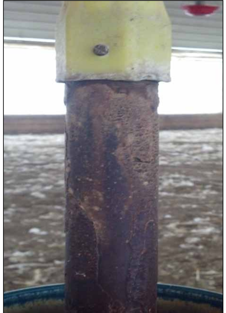
Without AquaKat - heavy scaling evident
