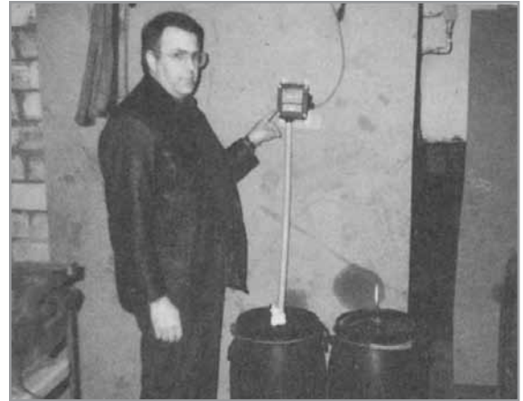
Figure 1: The Draeger measuring apparatus being used to measure the transformation of ammonia into ammonium in dairy manure following the introduction of penergetic g into the barrel.
